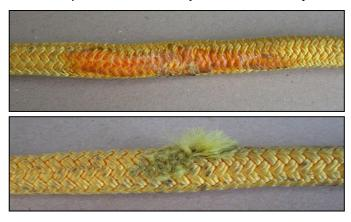
Inspection of the strops body reveals inconsistency in Diameter, Lumps/Bumps/Flat Areas with no external visible damage to jacket is probable indication of internal damage IE Shock Loaded, Broken Internal Strand/s
