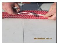
Form a loop of the nylon braid across the area to be repaired above where braid brought through the strop.
