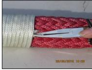
Draw the open end of the loop which pulls the loop to the centre of the whipping to lock in both ends.
