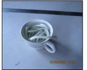
Soak nylon braid in hot water prior to repair, wet nylon braid will shrink when dry.
