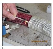
The excess braid can be neatly trimmed.
