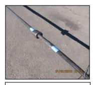
Heat Shrink sleeve one end to edge, masking tape protects fibres at ends.
