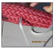
Insert braid through the Mongoose strop one end of repair.
