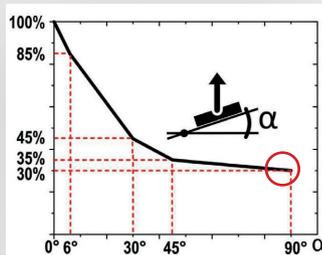
**Maximum load weight with 3:1 safety factor =  $320 \text{ kg} \times 100\% \times 30\% = 86.4 \text{ kg}$**
