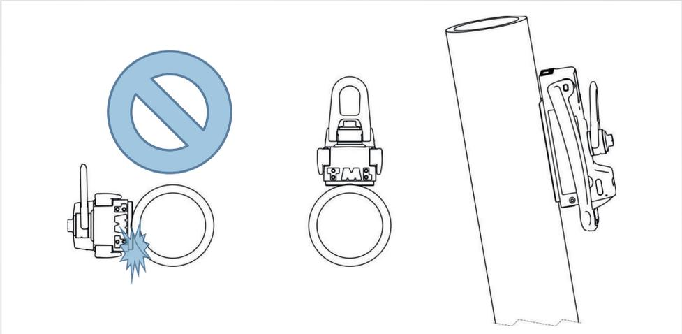
8. If the magnetic adhesion is sufficient and there is no deformation, you can continue the lift.
