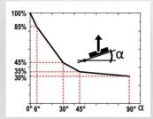
Maximum load weight with 3:1 safety factor = 360 kg x 100 % x 30 % = 108 kgMaximum load weight with 3:1 safety factor = 800 lbs x 100 % x 30 % = 240 lbs
