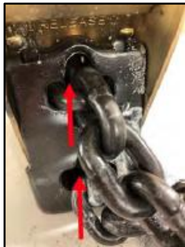
c) Through chain guard towards the chain wheel
