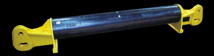
The Maxilug 25 allows users to create their own custom length, medium-lift spreader bar utilizing these heavy duty end units. Designed to accomodate readily available line pipe, Maxirig can supply the units as is or with various pipe lengths to facilitate lifts of varying dimensions up to 12 metres.
