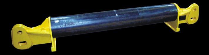
The Maxilug 50 allows users to create their own custom length, medium-lift spreader bar utilizing these heavy duty end units. Designed to accomodate readily available line pipe, Maxirig can supply the units as is or with various pipe lengths to facilitate lift spans from 2 metres up to 12 metres.
