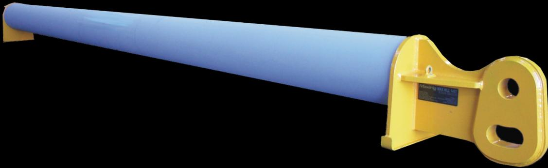
The Maxilug 145 allows users to create their own custom length, medium-lift spreader bar utilizing these heavy duty end units. Designed to accommodate readily available line pipe, Maxirig can supply the units as is or with various pipe lengths to facilitate lift spans from 2 metres up to 13 metres.
