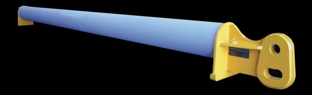
The Maxilug 400 allows users to create their own custom length, heavy-lift spreader bar utilizing these heavy duty end units. Designed to accomodate readily available line pipe, Maxirig can supply the units as is or with various pipe lengths to facilitate lift spans from 3 metres up to 13.5 metres.
